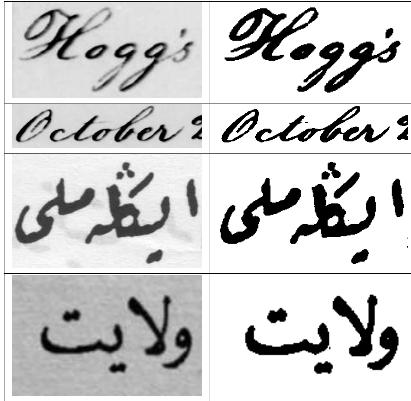
Figure 3.1: Original gray-scale images (left) used in word spotting task and their binarized versions (right) are provided.
