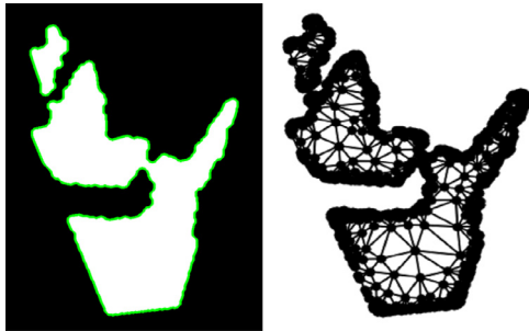
Fig. 7. Example triangulation of the navigable area. We preprocess the model image with erosion and dilation for refinement.
