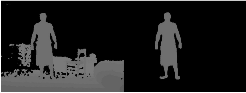
Fig. 8. The effect of depth map filtering. Notice the smoothed user boundary in the right image.
