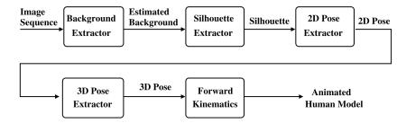
Fig. 1. The proposed framework for human motion capture from a single-view video sequence and animation using the motion capture data.
