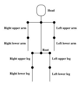
Fig. 2. The human body model used in the implementation.
