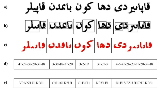
Fig. 10 Grouping recognized letters into words and mapping these words into ASCII characters.
