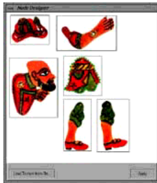
Figure 4: Node Designer Tool of the Hierarchy Editor; this tool is used to create the parts of an articulated character by using textures and polygons defined by using mouse.
