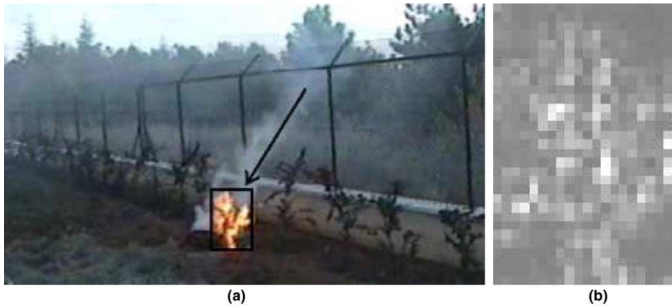
Fig. 6. (a) Fire, and (b) the absolute sum of spatial wavelet transform coefficients, |x_{lh}[k, l]| + |x_{hl}[k, l]| + |x_{hh}[k, l]| , of the region bounded by the indicated rectangle.
