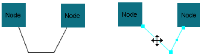
Figure 34 Bend point deletion; initially the edge has two bends (left); upon drag and release of the left bend, it is deleted to leave the edge with only one bend (right).
