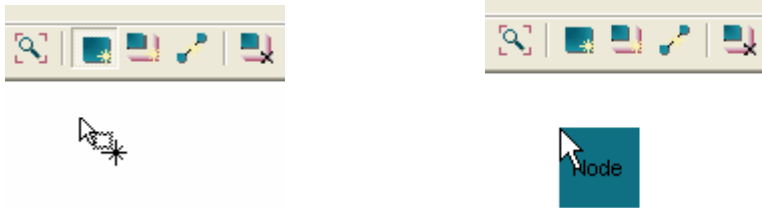
Figure 22 Create a node by simply clicking on the drawing canvas, where you would like your new node to be placed; before the creation (left) and after the creation (right).
