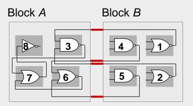
Cut  $c_a$ : four external connections
