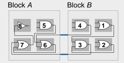
Cut  $c_{\rm b}$ : two external connections
