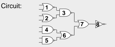
Partition the netlist into 2 equal parts (i.e. each part must have 4 gates) such that the # of edges between two partitions is minimized.
