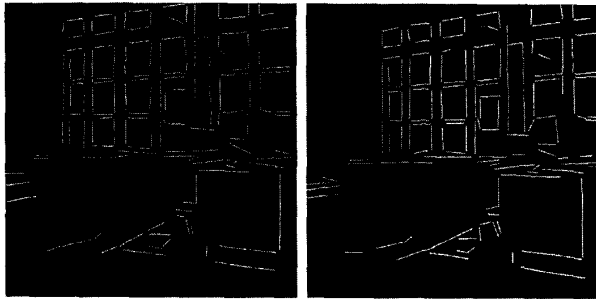
Fig. 4. Matching edge segments from a stereo pair of images.
