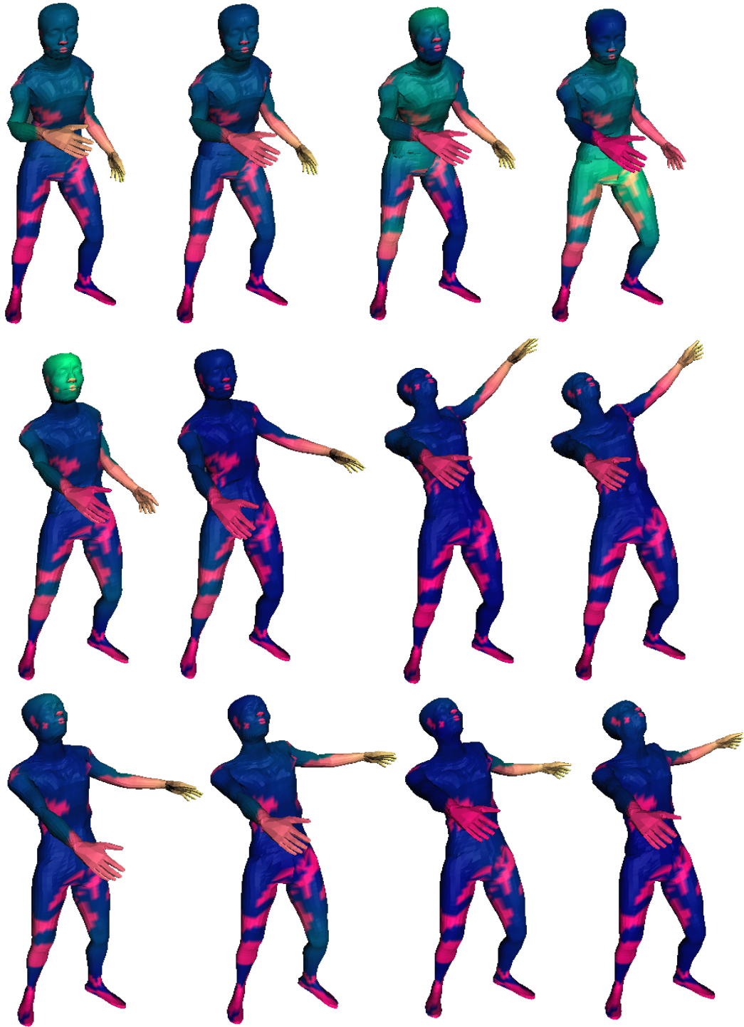
Figure 4.4: The results of oscillating motion detection on another motion capture sequence. The direction change threshold angle is taken as 90 degrees and we mark the vertices having variance between 2 and 6.
