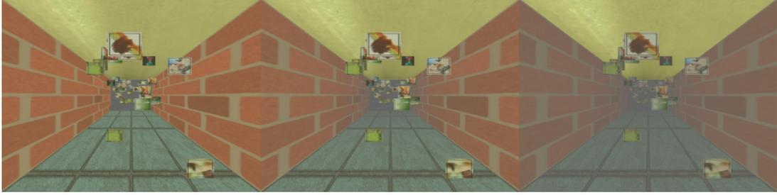
Figure 3.10: Effect of the fog rendering method. (Left: original scene, Middle: the scene with linear fog, Right: the scene with exponential fog)
