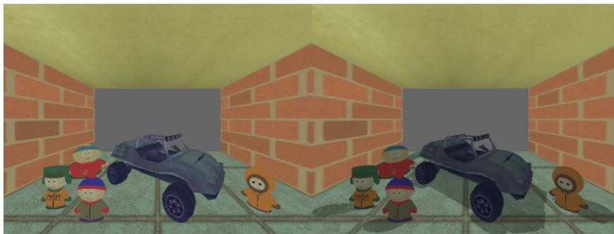
Figure 3.9: Shadow map method. (Left: original scene, Right: the scene with shadows)
