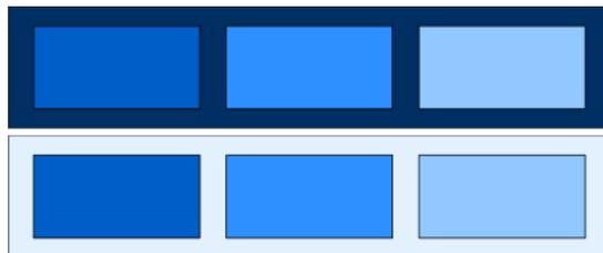
Figure 2.7: Relative brightness depth cue. (On the upper part, the brightest rectangle is perceived closest; on the lower part, the darkest rectangle is perceived closest.)
