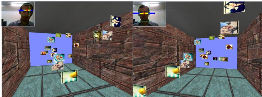
Figure 3.15: Demonstration of the face tracker in a camera application. (Left: The user looks at the scene from left. Right: The user looks at the scene from right.)
