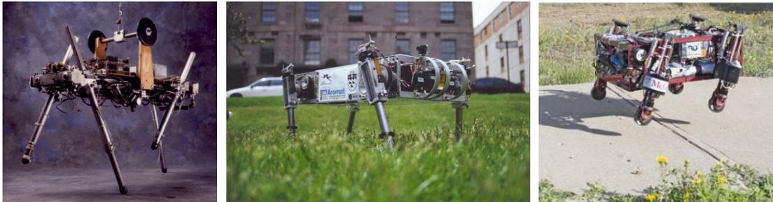
Figure 2.4: Raibert’s quadruped (left), SCOUT II platform (middle), PAW robot (right)
