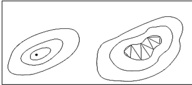
**Fig. 3.** TINs in an island-like situations should be handled with care.
