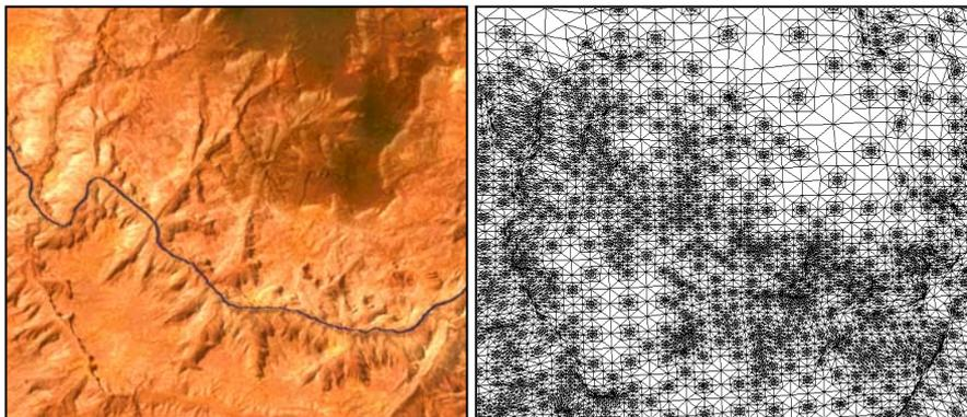
**Fig. 5.** *A simplified quadtree representing a particular terrain (Grand Canyon data obtained from the United States Geological Survey (USGS). Processing by Chad McCabe of the Microsoft Geography Product Unit.).*
