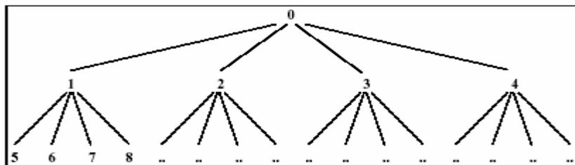
**Fig. 4.** Quadtree structure.
