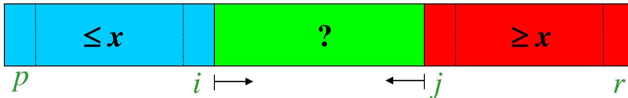
2. Lomuto's algorithm: Partitions around the last element of subarray ( $pivot = x = A[r]$ )
