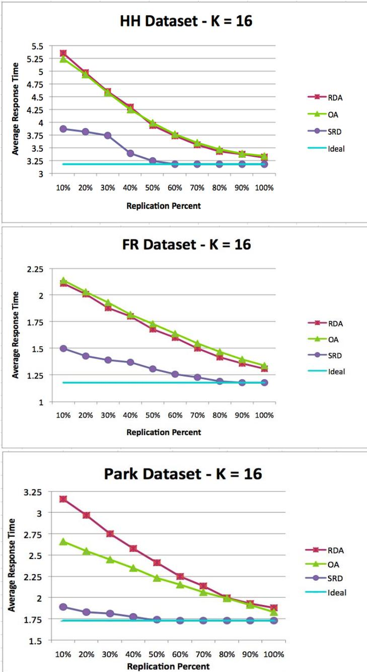
Fig. 1. Comparison of average response time qualities of the Random Duplicate Assignment (RDA), Orthogonal Assignment (OA), and Selective Replicated Declustering (SRD) schemes with increasing replication for  $K = 16$  disks
