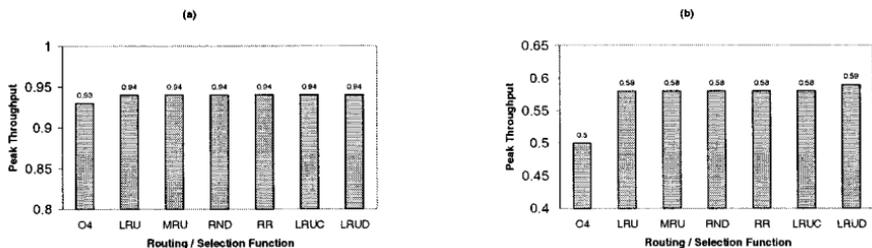
**FIG. 21.** Peak throughput for the oblivious routing and adaptive routing with different selection functions on a 16-node system with random traffic pattern for (a) 128-byte messages and (b) 4096-byte messages.
