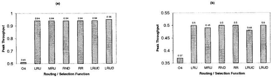
**FIG. 23.** Peak throughput for the oblivious routing and adaptive routing with different selection functions on a 128-node system with bit-reversal traffic pattern for (a) 128-byte messages and (b) 4096-byte messages.
