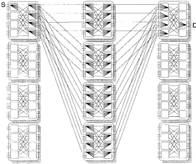
FIG. 4. A 128-node SP switching network. A subset of the entire set of links is shown.
