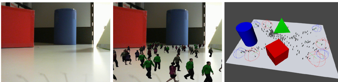
Figure 1: An example AR environment. Left: the real environment with simple geometric primitives. Middle: the view the user sees through the AR display. Right: the collision mesh and synthetic agents in virtual environment. The red and blue wireframe hemispheres represent the locations where the agents are created and destroyed.
