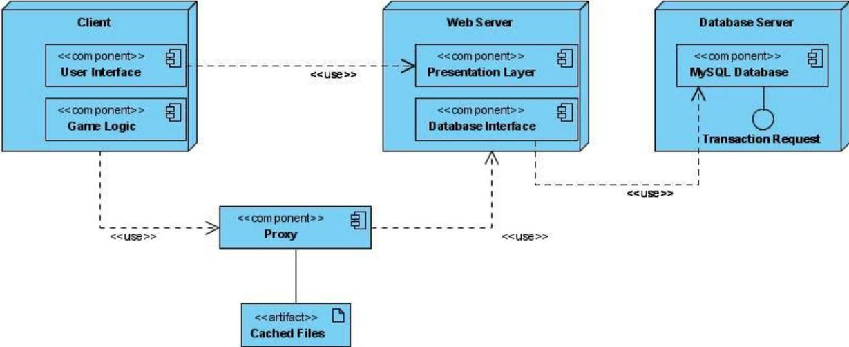
**Figure 3.** Client-Server System Deployment Diagram
