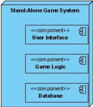
**Figure 2.** Stand-Alone System Deployment Diagram
