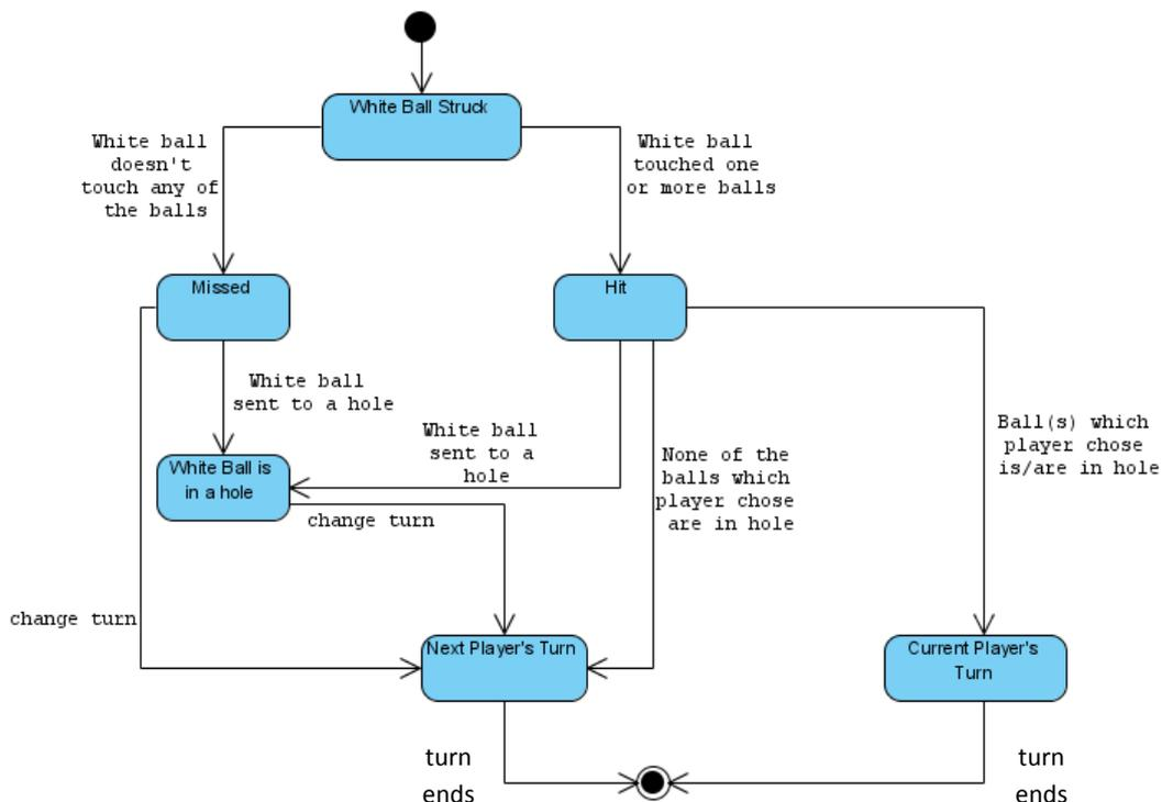
Figure 7: Ball State Diagram
