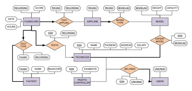
It is not possible to express that the tests on a plane must be conducted by a technician who is an expert on that model because the constraint is on the Entities. We can do this by dividing different expertise of technicians and the models but this would limit adding new models and expertise types of the technicians.
