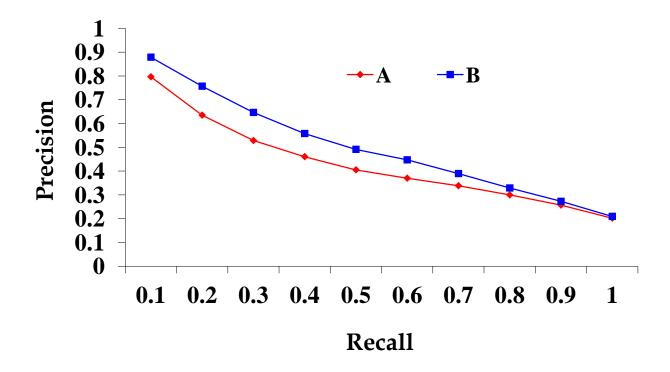
Using precision-recall graph we can compare two information retrieval systems. The curve closest to upper right corner of graph indicates better results.
