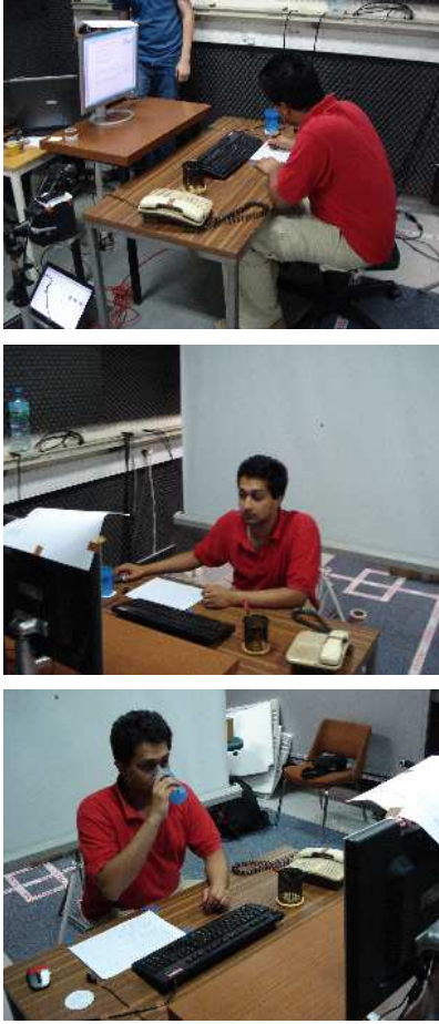
Fig. 1. The pilot setup, shown during one of the recordings. The frontal cameras are mounted on the display, and the side camera is mounted on a pod to the left of the subject.
