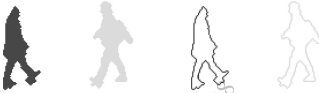
Fig. 6.2. Detected regions and silhouettes. Left: Detected and labeled object regions. Right: Extracted object silhouettes.
