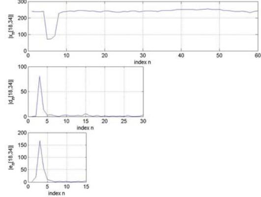
Fig. 2. Temporal history of the pixel [18,34] in time (top). Wavelet domain subsignals  $d_n$  and  $e_n$  exhibit a stationary behaviour for  $n > 8$ .
