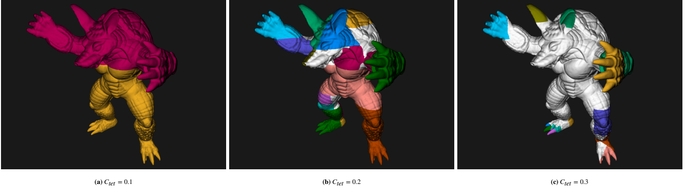
FIGURE 4 Tetrahedralizations of BTH constructed using different C_{tet} values. Different tetrahedralizations are colored differently. Gray color is used for faces in the BVH structure.
