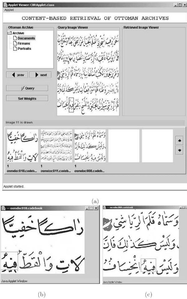
Fig. 11. Query example. (a) Document image where the query image is specified by a rectangle. (b) First retrieved document with 1 match. (c) Third retrieved document with one match (second retrieved document is the query document itself.). This query example also shows the scale invariance property.
