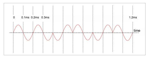
A digital bit stream that is coming to a **BPSK** modulator is modulated over the air and the above pattern is observed for the modulated signal in the air. The data bit-rate coming to the modulator is 5000 bps. Which data bit pattern is respresented with the signal above? (Namely, what is the data bit sequence encoded into the signal above?).
