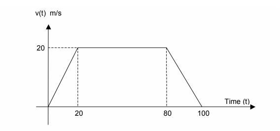
A car is traveling along a street with velocity v(t) as shown in the figure. The received signal experiences multi-path Rayleigh fading on a 900 MHz CW (continues wave) modulated carrier. Assume  $\rho$ =0.1 and ignore large-scale fading affects.
