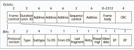
Figure 3. Standard IEEE 802.11 frame format.
