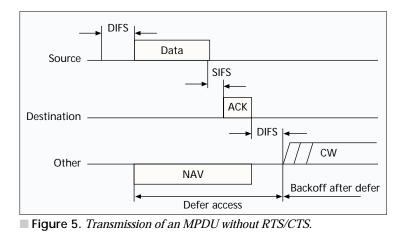
tion, payload, and a 32-bit CRC. The duration field indicates the amount of time (in microseconds) after the end of the present frame the channel will be utilized to complete the successful transmission of the data or management frame. Stations in the BSS use the information in the duration field to adjust their network allocation vector (NAV), which indicates the amount of time that must elapse until the current transmission session is complete
