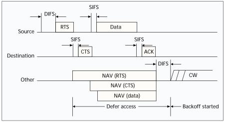
Figure 6. Transmission of an MPDU using RTS/CTS.
