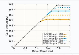
Figure 14. Average MSDU length effects on data throughput.
