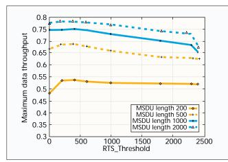
Figure 12. RTS\_Threshold effects on data throughput.
