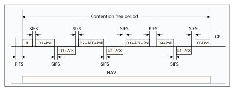
Figure 9. PC-to-station transmission.
