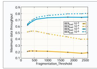
Figure 13. Fragmentation\_Threshold effects on data throughput.
