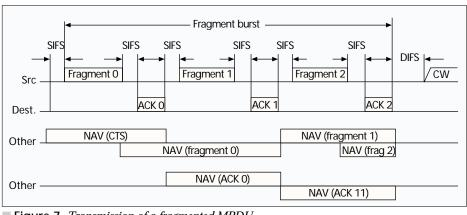
Figure 7. Transmission of a fragmented MPDU.
