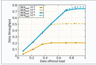
Figure 11. Burst error effects on data throughput.
