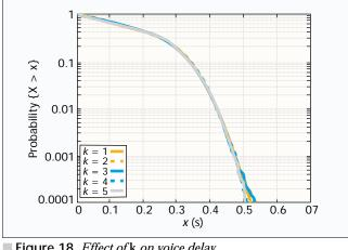
Figure 18. Effect of k on voice delay.
