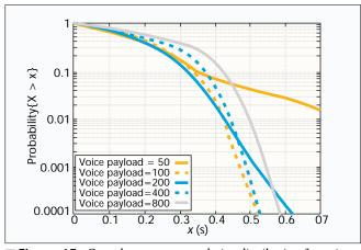
Figure 15. Complementary cumulative distribution for voice delay.
