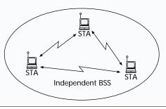
Figure 1. Sketch of an ad hoc network.
