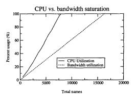
**Figure 8.** An example of a CPU-bound configuration of INS. The Pentium II processor is saturated well before a 1mbit/s link. Numbers are shown with refreshes happening every 15 seconds.
