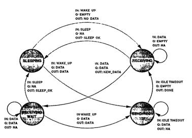
Figure 1. Slave (Base Station) Protocol State Diagram
