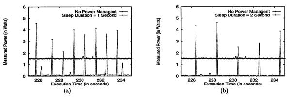
Figure 4: Power Consumption During a Sample Idle Period
