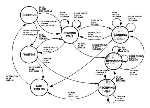
Figure 2: Master (Mobile Host) Protocol State Diagram
