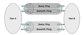
Fig. 4. Two OWRCs between two peers, which enable each peer to request service from the other.
