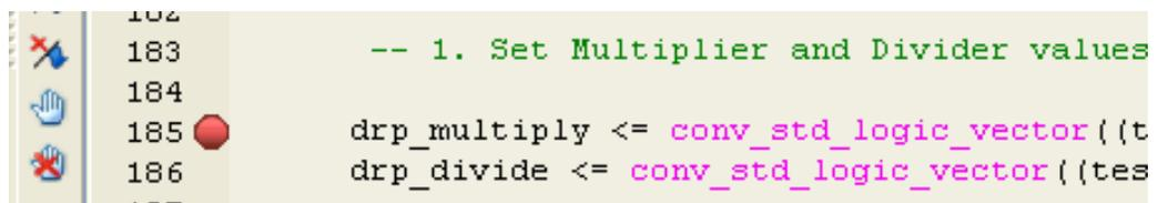
Figure 4-47: **Setting a Breakpoint at Line 185 in drp\_demo\_tb.vhd**
