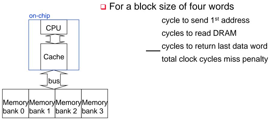
Number of bytes transferred per clock cycle (bandwidth) for a single miss is
