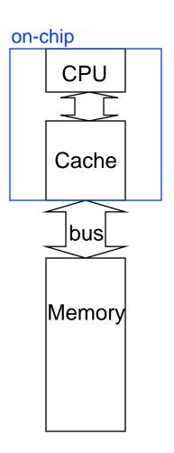
If the block size is one word, then for a memory access due to a cache miss, the pipeline will have to stall the number of cycles required to return one data word from memory
