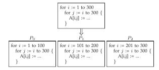
Fig. 4. Data parallelization of a loop nest.
