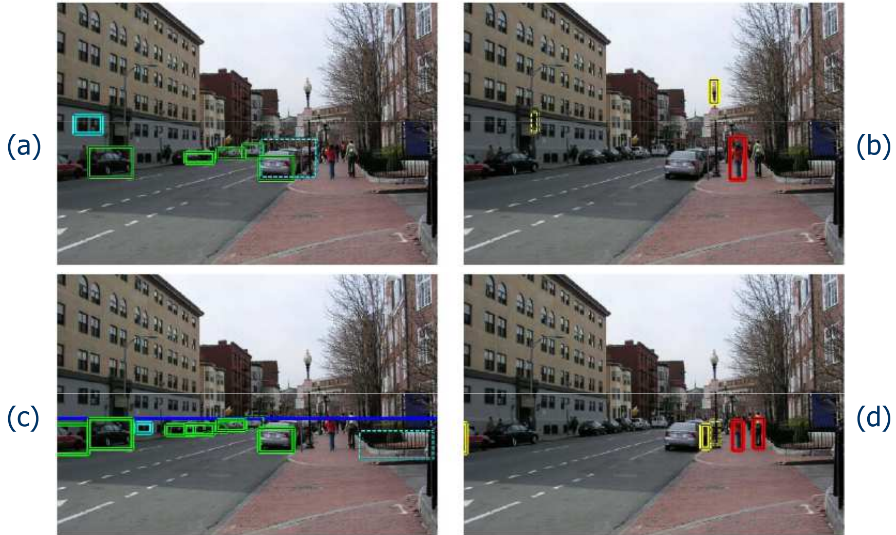
Putting objects in perspective: Car (a) and pedestrian (b) detection by using only local information. Car (c) and pedestrian (d) detection by using context. (Hoiem et al. "Putting Objects in Perspective," CVPR, 2006)
