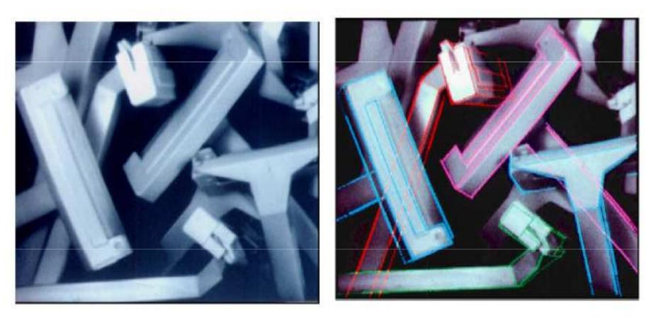
"Project" model into image and "match" to lines (solving for 3D pose).
