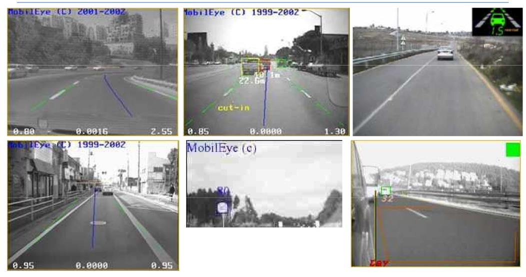
Lane departure warning, collision warning, traffic sign recognition, pedestrian recognition, blind spot warning
