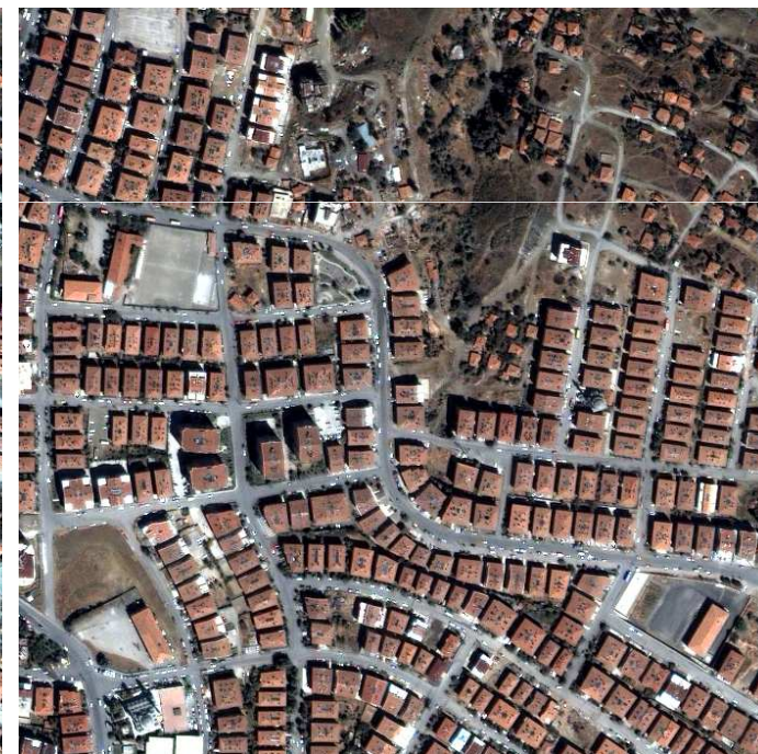
Histogram stretching by removing 2% percentile from each individual band/channel
