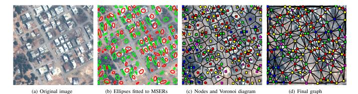
Figure 1. Feature extraction and graph construction steps. MSER+ and MSER- ellipses are shown as green and red, respectively, in (b). The color and symbol of a node in (c) and (d) represent its label after k-means clustering.
