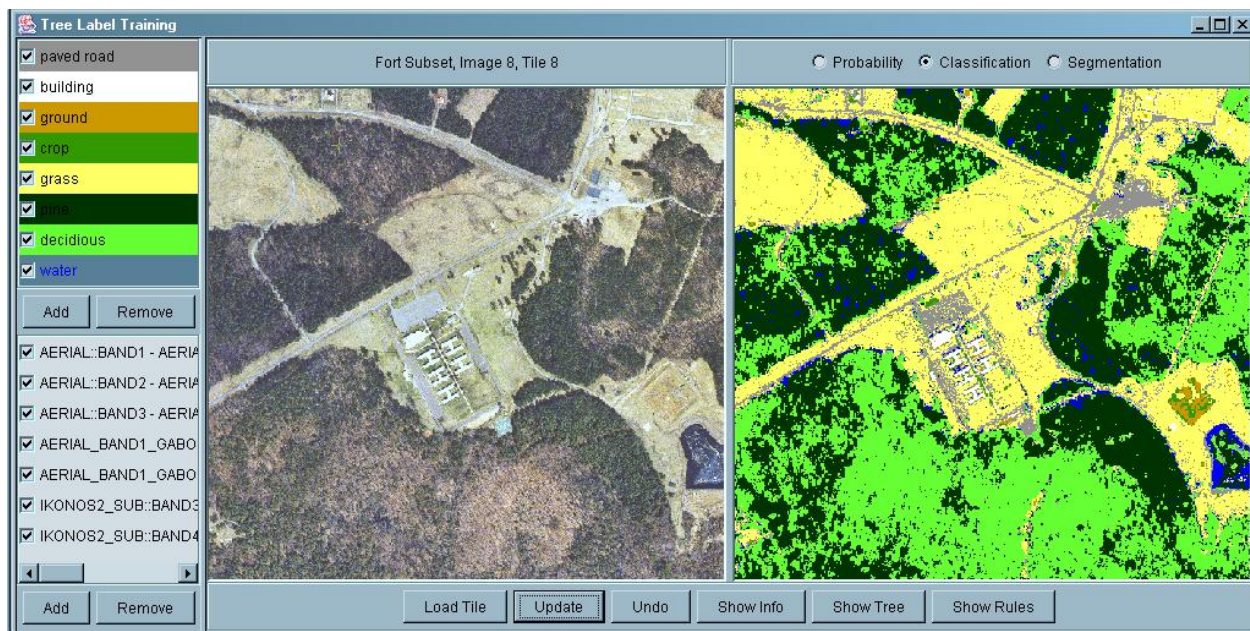
Figure 2: Graphical user interface for training classifiers. The panel on top-left shows the land cover/use classes defined by the user. The user can add new classes or remove existing ones, and can also change the color of a class. The panel on bottom-left shows the data layers used in training. The user can add or remove layers at any time of the training process, and examine the difference in classification results using the previously given training examples. Double-clicking on a data layer shows that layer on the left image panel. The “load tile” button loads a new image for training and/or classification. The “update” button shows the probability map for an individual class or the classification map for selected classes on the right image panel. The “undo” button removes the latest example submitted to the classifier. The “show info” button displays information about the trained classifier. The “show tree” and “show rules” buttons open the tree and rule displays, respectively.
