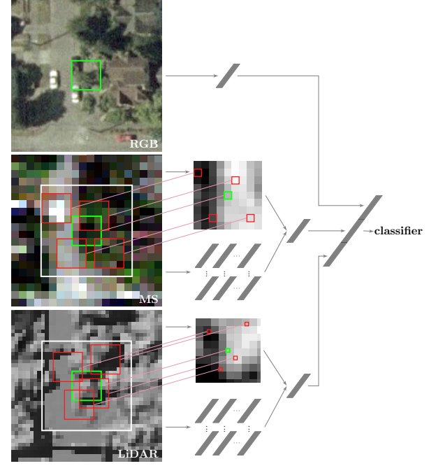
Fig. 1. Attention-driven representation of multisource data with imperfect pixel-level alignment. The RGB image, where a 25 \times 25 pixel region (shown as green) centered at a verified ground truth tree location, is considered as the reference source. The corresponding regions in the MS and LiDAR data occupy 4 \times 4 and 8 \times 8 pixels (also shown as green), respectively. The proposed multisource region attention network evaluates candidate regions (shown as red) sampled within a larger neighborhood (shown as white) around the expected object position, computes attention scores (shown as a grayscale map) that represent the confidence about each candidate containing the object, uses these scores to form the attention-driven multisource representation .
