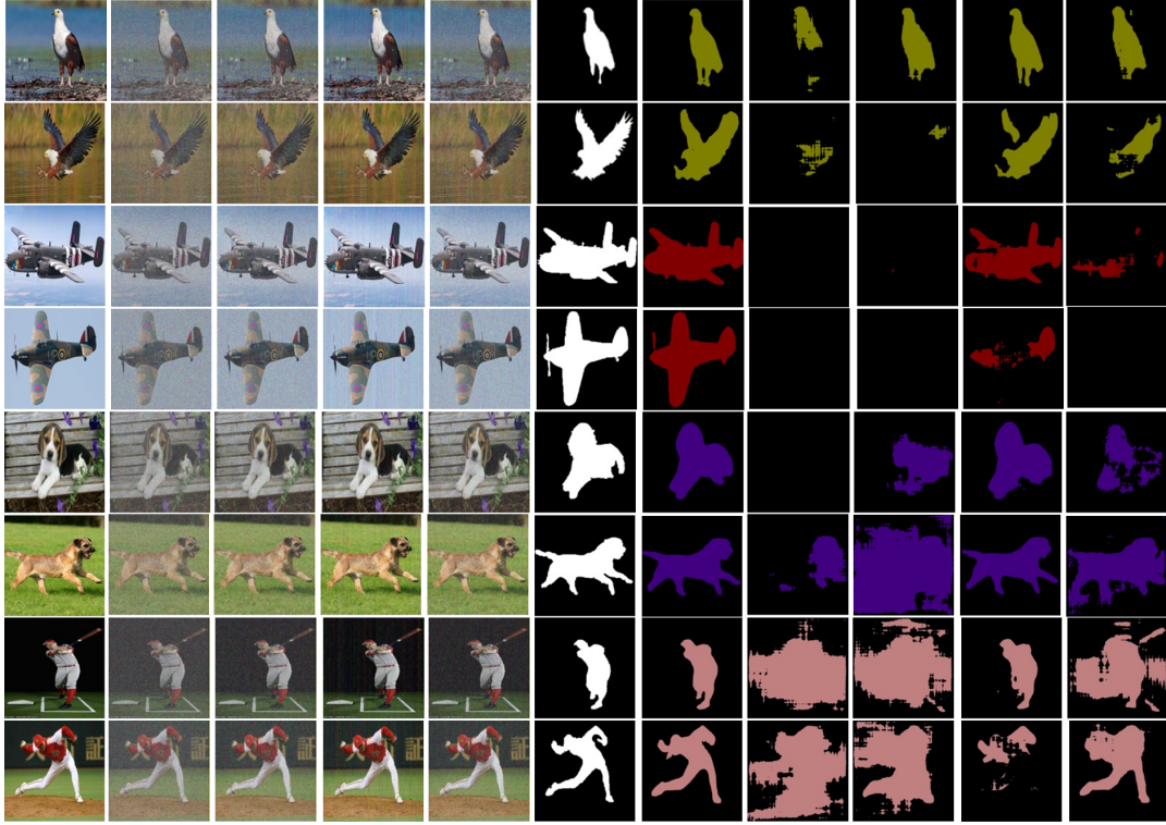
Fig. 5: Qualitative results obtained at different system parameters for sample images. The 1st column shows sample (input) images. The 2nd, 3rd and 4th columns show the results obtained at 5dB, 10dB and 15dB SNR values respectively (where UAV velocity is 41.6 m/s). The 5th column shows the result, when SNR=15dB but the UAV velocity is set to 55.4 m/s. The 6th column shows the ground truth segmentation, the 7th column shows the segmentation results of MobileNetv2, when there is no noise and no Doppler effect. The 8th, 9th, 10th and 11th columns show the offloaded segmentation results obtained for the images as shown in the 2nd, 3rd, 4th and 5th columns, respectively.
