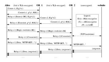
Figure 1: Alice builds a two-hop circuit and begins fetching a web page.
