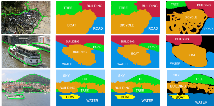
Figure 19: Example results where context improved the categorization accuracy. Left to right: original segmentation, categorization w/o contextual constraints, categorization w/ contextual constraints, ground truth.
