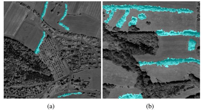
**Fig. 4.** Example results for final detection based on morphological shape analysis.
